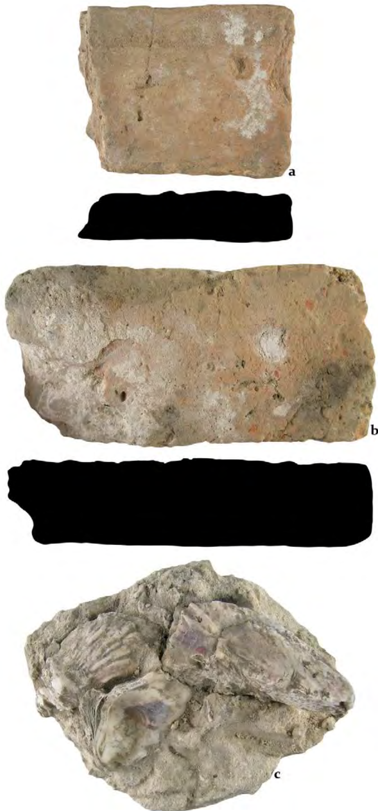
Figure 3-57. Structural materials: (a-b) French-style bricks with drawn profiles (Area 3, FS 1018); (c) tabby mortar with oyster shells (Area 6, FS 980) (all half size).
