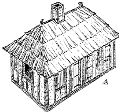
Figure 6-4. Drawing of a poteaux sur sole (post on sill) structure at Old Mobile (1MB94) by Philippe Oszuscik, based in part on archaeological remains.
