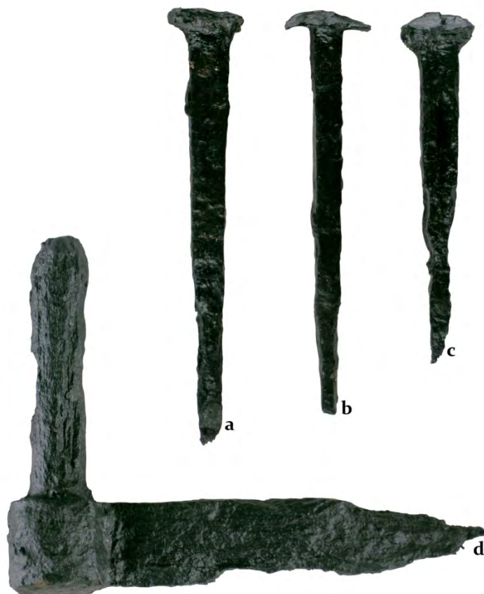
Figure 3-56. Iron hardware: (a-c) wrought rosehead nails (Area 3, FS 1017; Area 7, FS 294 and 892); (d) shutter pintle (Area 1, FS 1205) (all actual size).
