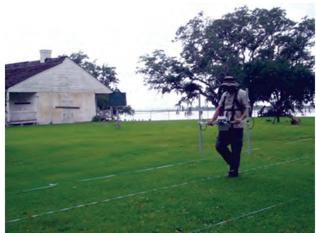
Figure 2-1. Survey transect using gradiometer.
